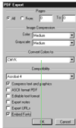
In the PDF Export dialog box, convert colors to CMYK, select Embed Fonts, and set other options appropriate for the PDF file you're creating
